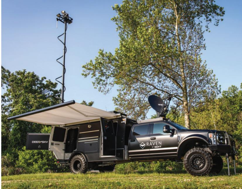
The Raven is a mobile command center that collects and distributes mission-critical information in operational environments. Powered by artificial intelligence and machine learning systems, the Raven can filter information to enable data-driven decisions that can be disseminated to first responders, analysts and decision-makers in real time, whether connected or disconnected from the enterprise.
